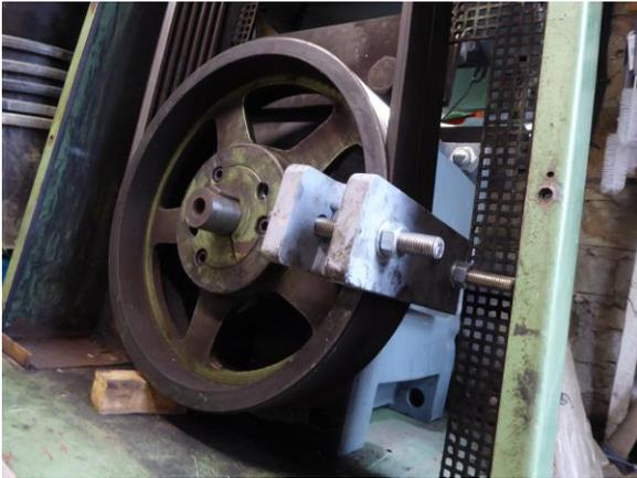
While LSP was working on the sluice gate, the river was still flowing through Archie as the gate was effectively fully open. Allowing Archie to run free under these conditions would have been exceptionally dangerous so some considerable thought went into ways of preventing this. The drive to the generator had to be clamped to stop the screw turning but still allow the excess water to flow over the top. How was this done? Take a look at the picture!
